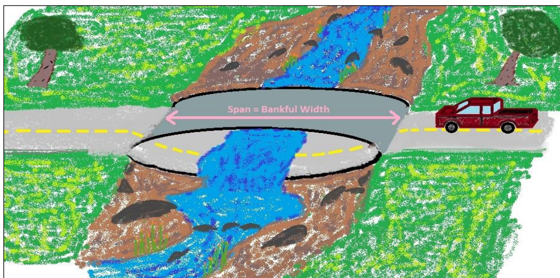
Figure 6. Depiction of low-water crossing modeling in FishXing with large horizontal ellipse culvert.
