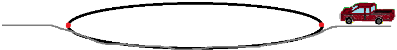
Figure 131. Profile depiction of horizontal ellipse culvert (black), vertex points (red), and low-water crossing (grey) margin differences.
